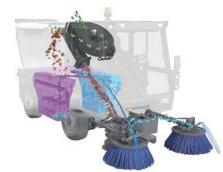
The 2-brush system with independently controlled circular brushes guarantees absolute mobility in every sweeping situation. Two stable brush arms with integrated buffers allow sweeping widths of up to 2,900 mm. Swingo 200<sup>+</sup> | 3-Brush
