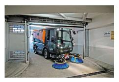
A lowerable running gear (optional) simplifies driving in multi-storey car parks and low entrances. The chassis can be lowered by around 70mm at the push of a button and the system levels itself automatically.
