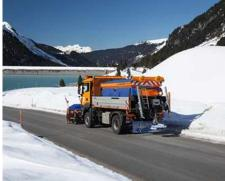
The Stratos 50 is a mounted spreader with a hopper capacity of 5 m<sup>3</sup>.
