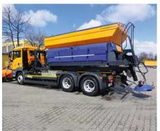
The Stratos 100 is a spreader with a hopper capacity of 10 m<sup>3</sup>.
