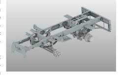
driving even in bad road and weather conditions. The Cleango 500 has the highest payload in its class - up to 6,600 kg thanks to robust suspension, high axle loads and twin tyres on the rear axle. A large steering angle of 68°, combined with the short wheelbase of 1.850mm, allows optimum manoeuvrability and an extremely tight turning circle.
