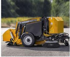
The MSH 150 has a steel hopper with 1.5  $m^3$  capacity.
