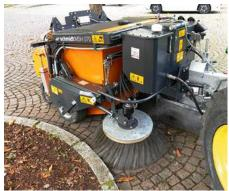
The MSH 070 has a steel hopper with 0.7  $\ensuremath{\mathsf{m}}^3$  capacity.
