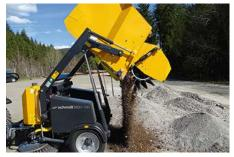
The MSH towed sweeper series has a steel hopper with a capacity of  $0.7 \text{ m}^3$  and a discharge height of 1,500 mm for the MSH 070 version and a capacity of 1.5 m<sup>3</sup> and a discharge height of 1,800 mm for the MSH 150. In each case, the hopper is tipped hydraulically at the back.
